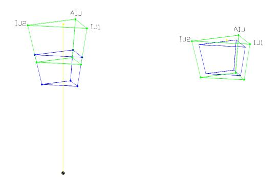
On top of that, we still need to re-locate the blue vertices so they line up with the bottom green ones The line-up would involve local scaling. However, since our tetrahedron is irregular, it is not a simple task to find the base point (centre) of this tetrahedron to enable this scaling. Nevertheless it led me to explore this issue of finding the proper midpoint of the tetrahedron. First of all, what is the midpoint of a triangle?
